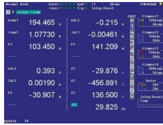
Example of DC voltage, current, and power at three points and conversion efficiency measurement.
