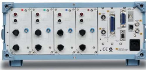
Rear panel (4 input elements and options)
