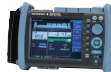
Optical Loss Test Set AQ1100
